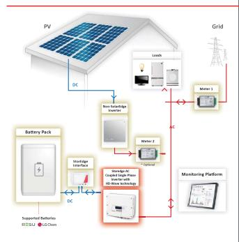
\* Optional - needed for full system monitoring: consumption, self-consumption and inverter production
